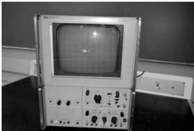
**Figura 5** – Painel Frontal Osciloscópio HP 143S Display Section.
